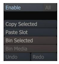
You can disable individual Slots so that they will be skipped for playback when the Construct is loaded into the Player. To disable a Slot you can use the **Enable** toggle button. When a Slot is disabled, the icon at the bottom left of the slot turns red. When you have multiple Slots on the CONstruct disabled you can quickly enable them by activating one of the disabled Slot and then select the **All** button before clicking the **Enable** button.
